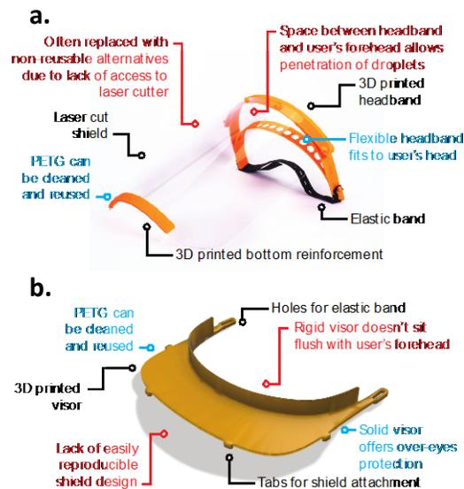
**Figure 1.a.** A photo of the Prusa headband design and **b.** a rendering of the Budmen and Columbia visor design.
