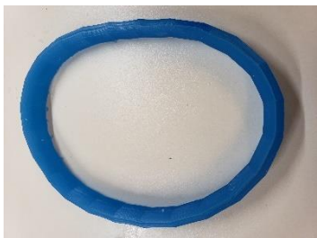
SILICONE GASKET (molded in-house)
