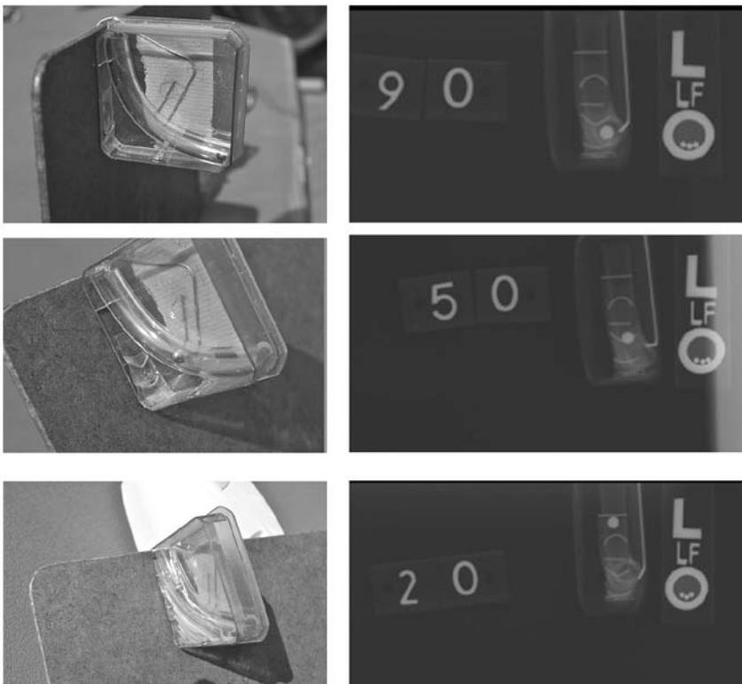
The clear plastic cylinder allows the ball to roll freely, resulting in visualization that verifies position. The sides are flat to allow consistent flush contact with the cassette. The metal clips are cut and taped to the cylinder in 10° increments (0°-90°) to differentiate inclination angles. A serpentine-shaped clip suspended the device on a cassette (see **Figure 2**).
