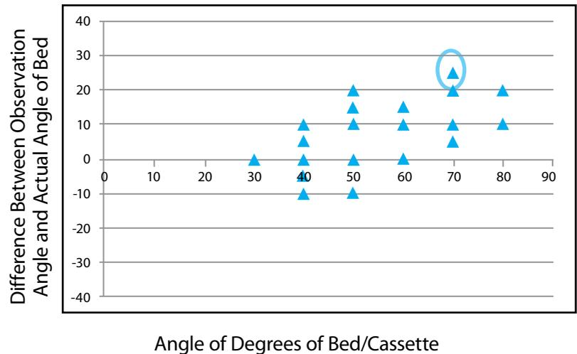
**Figure 5.** Summary of actual inclination angles and radiologist estimates on 27 patients. The largest error was  $25^\circ$  (circled); the radiologist estimated the angle as  $45^\circ$  when the actual angle was  $70^\circ$ .
