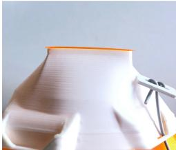
Ensure the brimmed lip of the TPU soft shell extends above the top lip of the PLA/PETG hard shell. ATTN: the seal of the tpu will still work if the brim has become loose or removed over time.
