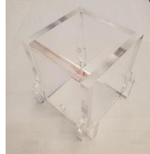
**Figure 2:** Abrasion testing box is shown (A) unassembled and (B) fully assembled.
