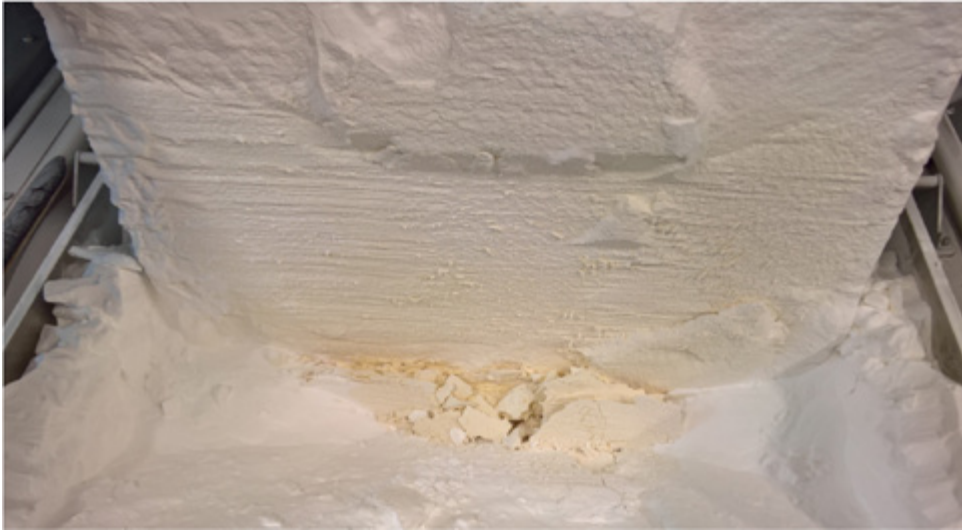
Example of brown powder in an HP Multi Jet Fusion printed bucket
