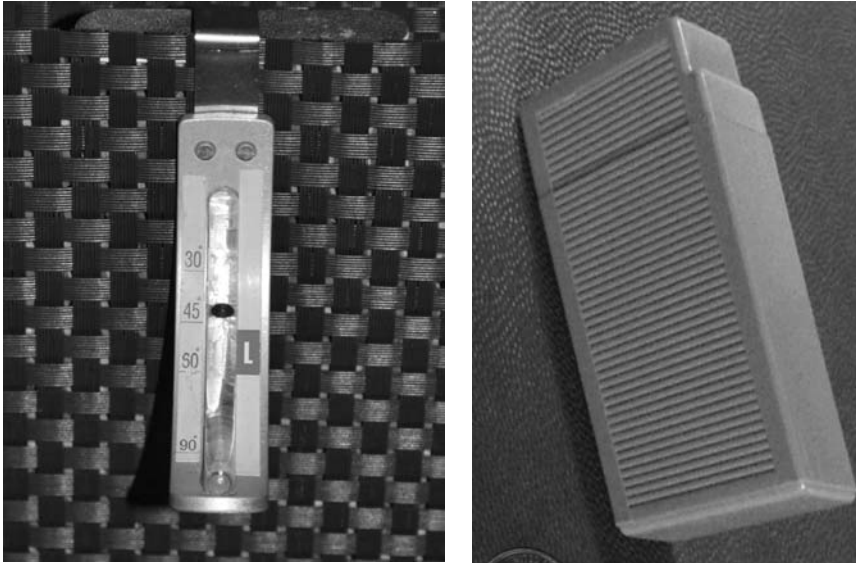
Figure 7. Photos of recently manufactured prototype UpRight markers that will be available commercially soon. The image on the right (A) shows the ball just under 45°. The marker on the left (B) has a radiopaque pendulum that indicates angle and has yet to be tested.
